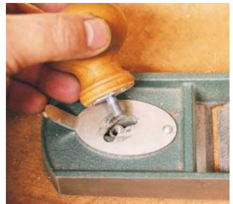
▲ A simple cam adjuster alters the mouth opening
